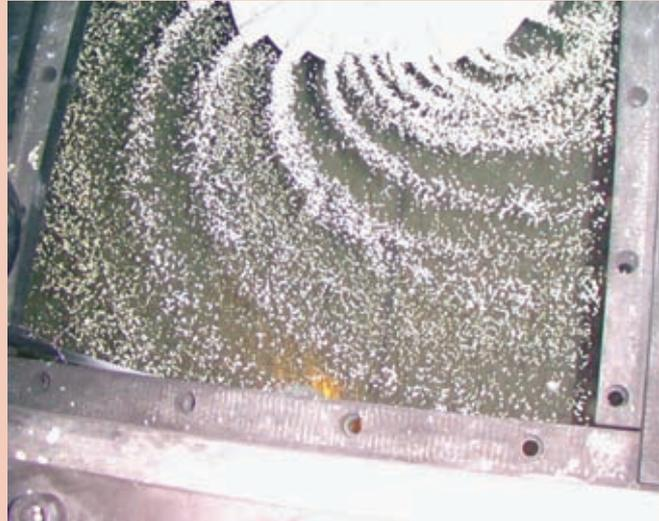
slump to a more dense structure. At end-of-run (EOR), a sock loaded bed will often have a pressure drop equal to that of a dense loaded bed. Dense loading fills a reactor with less open volume in the catalyst beds.
